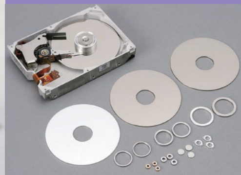
(JWP,FBB) aluminium substrates and spacer rings for computer (HDD)
